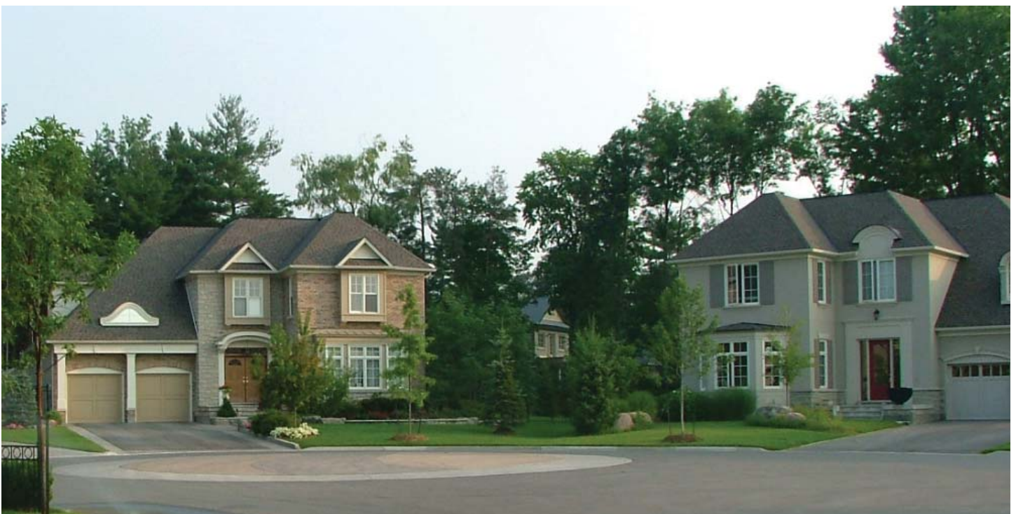
Figure 39 Locate driveways away from centre viewpoint to create visually attractive T-intersection and cul-de sac terminus views
