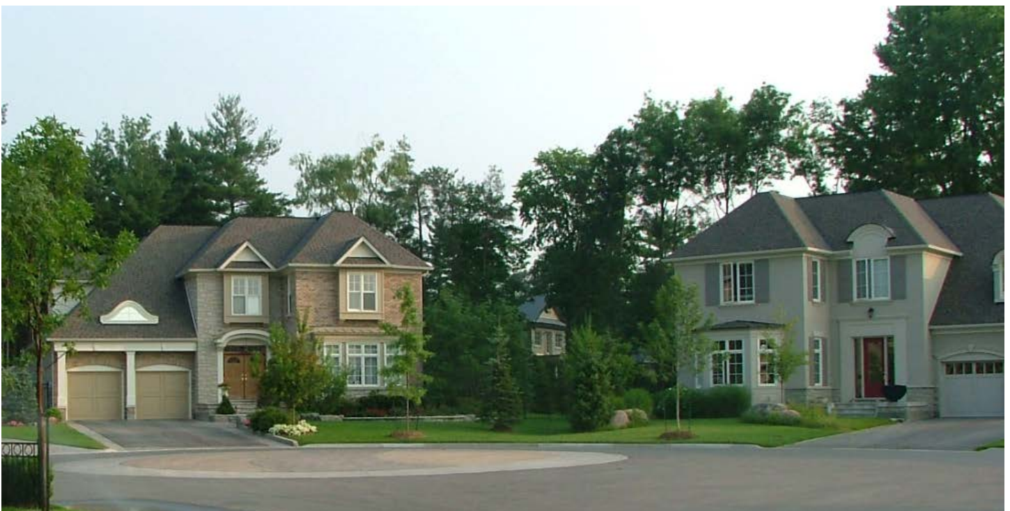
Figure 41 - Locate driveways away from centre viewpoint to create visually attractive T-intersection and cul-de-sac terminus views
