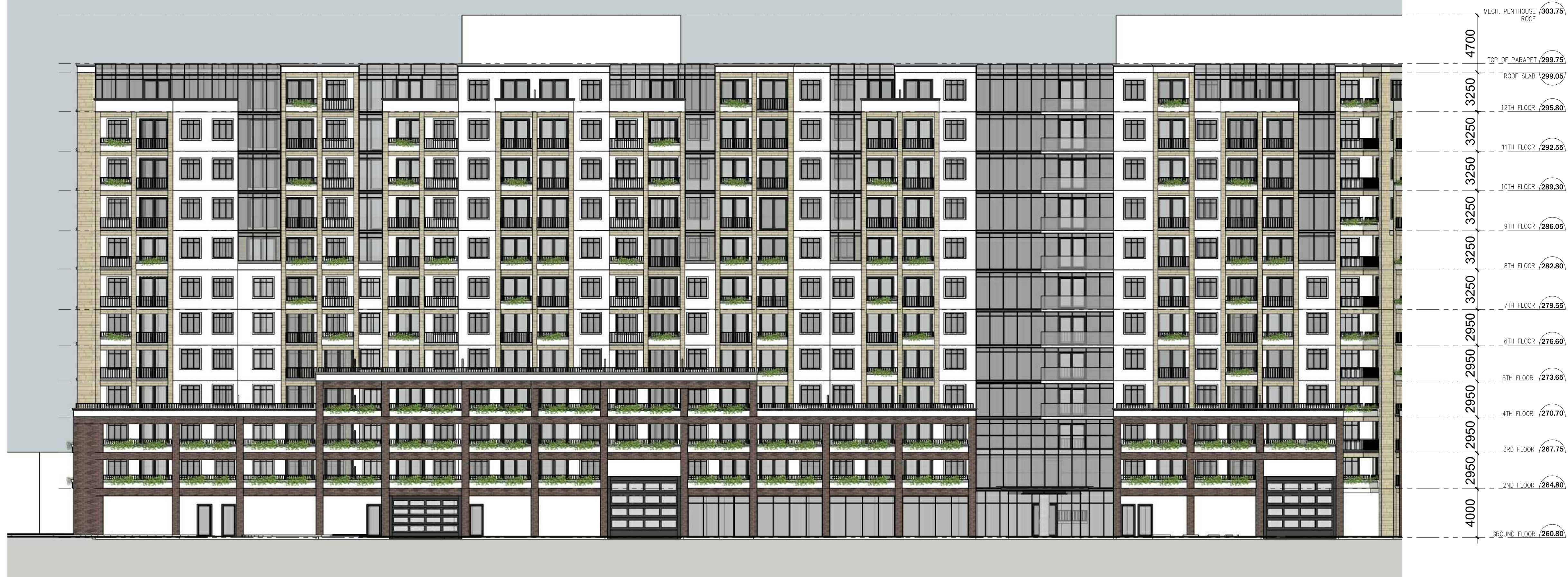
BUILDING - 1&2 _ NORTH ELEVATION _ SCALE 1:200
