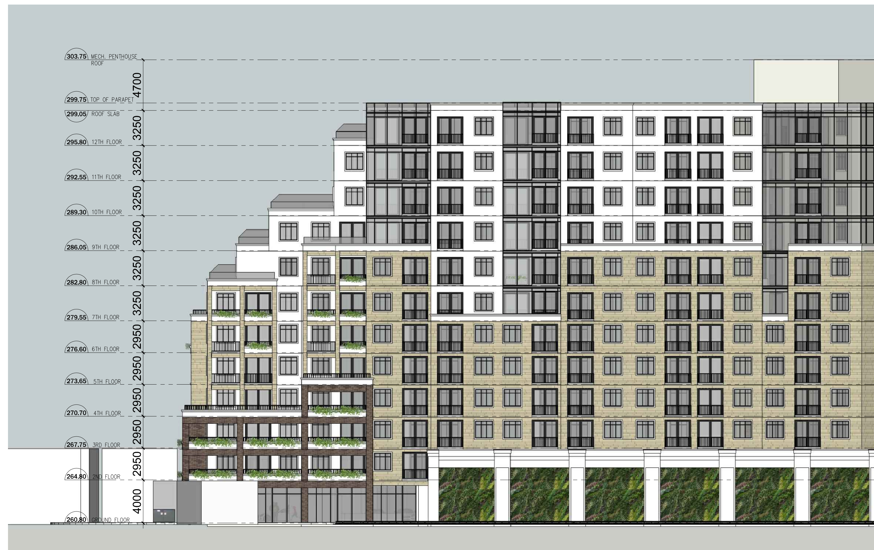
BUILDING - 2 _ WEST ELEVATION _ SCALE 1:200
