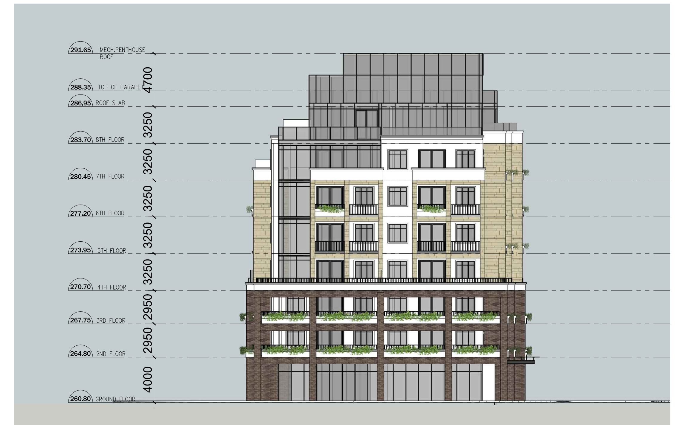
BUILDING - 3 _ NORTH ELEVATION _ SCALE 1:200
