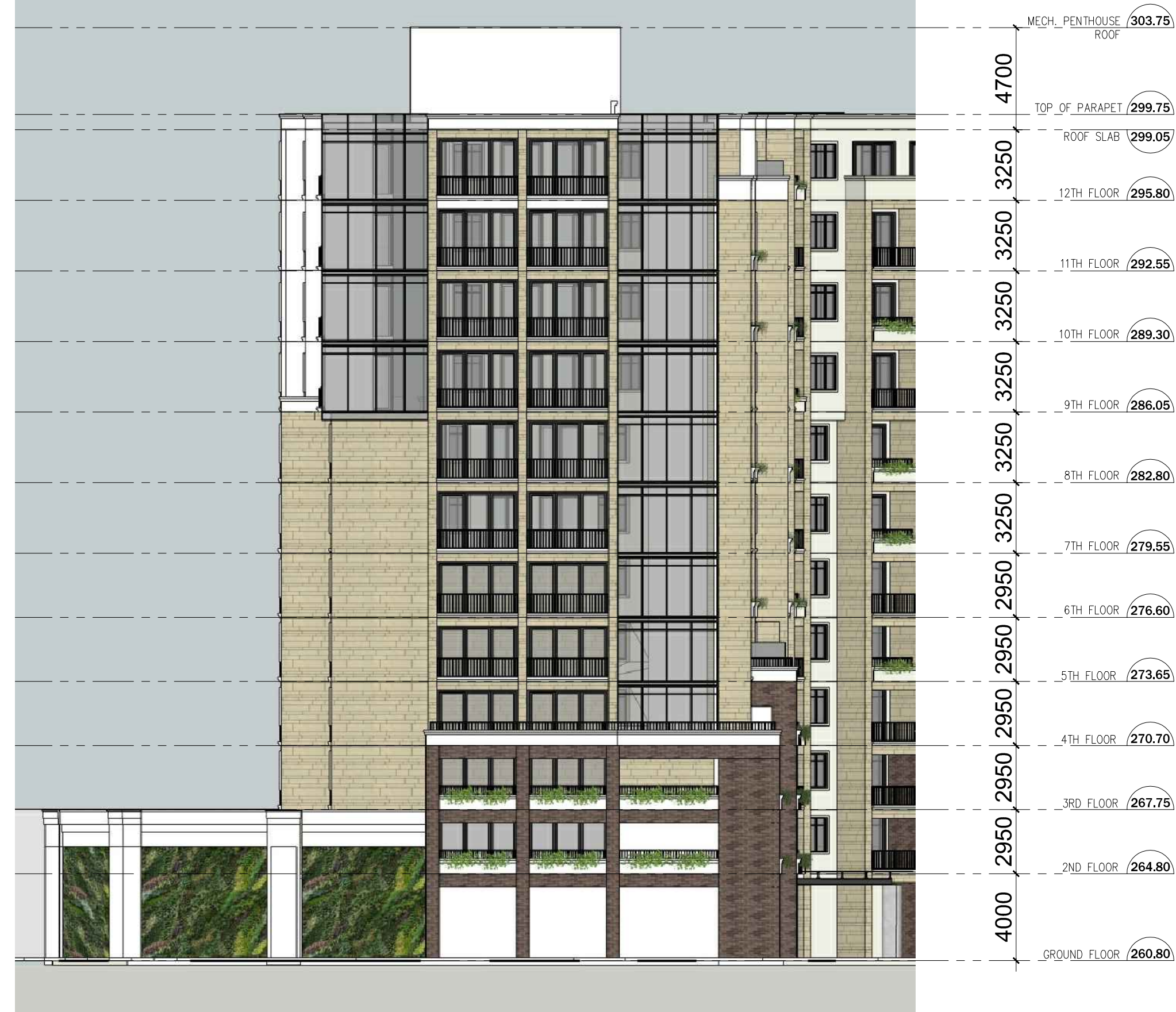
BUILDING - 1 _ EAST ELEVATION _ SCALE 1:200
