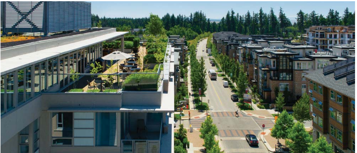
When building elevations can be seen from adjacent streets, massing should be broken up through building projections, colours, and certain architectural styles.
