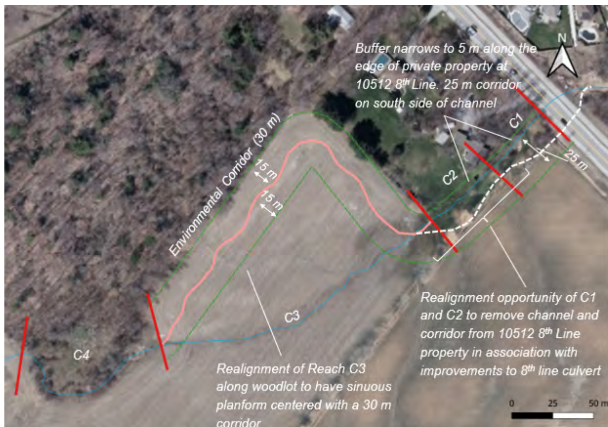
Figure 1: Plan view of the proposed realignment of reach C3, centered along a 30 m-wide environmental corridor contiguous with an existing woodlot.
