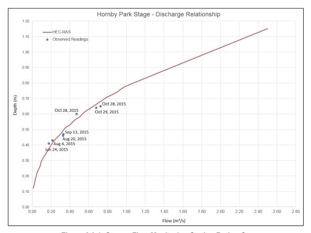
Figure 2.3.1: Stream Flow Monitoring Station Rating Curve
